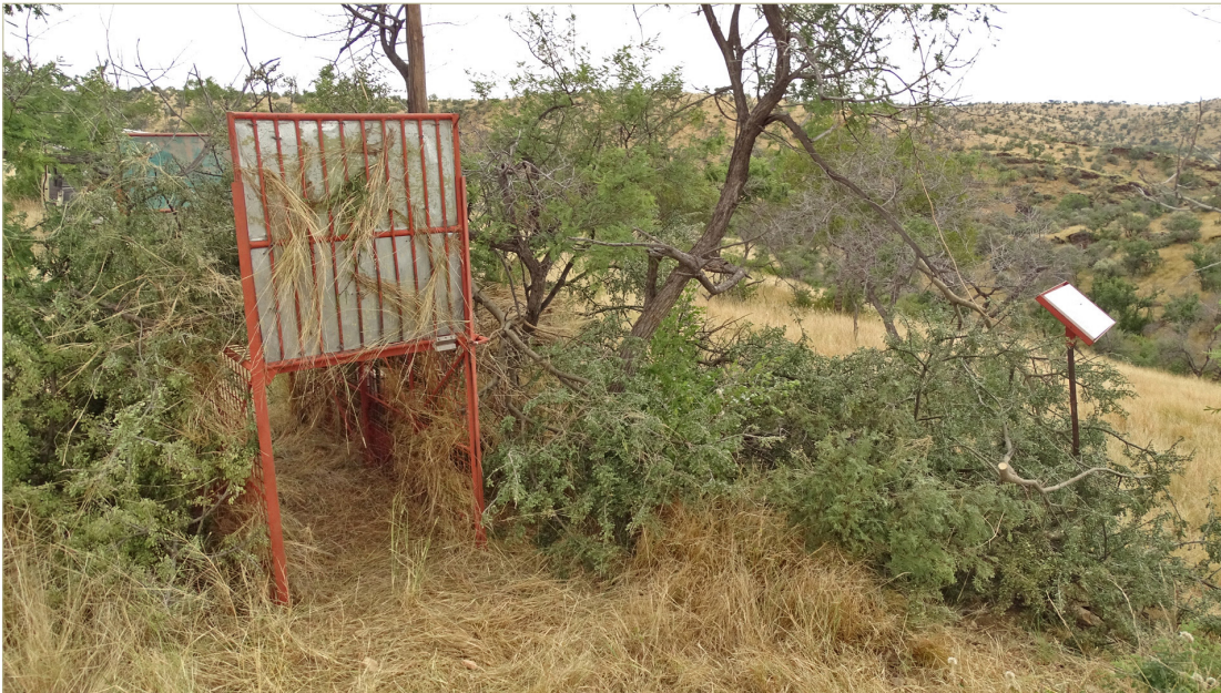
Figure 6: Electronic traps monitored by GSM/GPRS or satellite communication are used to efficiently capture free-ranging leopards. Photo credit: Ruben Portas
